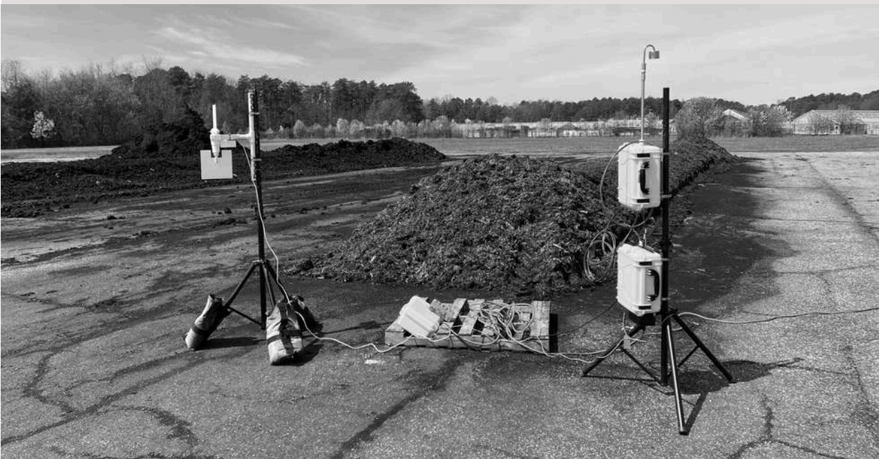
Above Image of the AeroExplorer Trace Gas sampling system configured for sampling by wind direction
