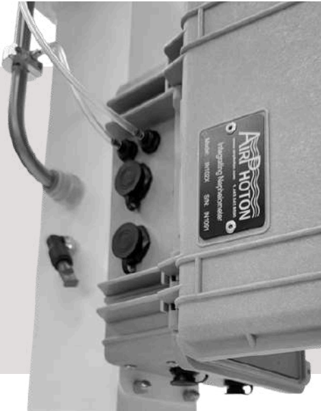
Dual pressure taps in inlet to provide accurate flow monitoring
